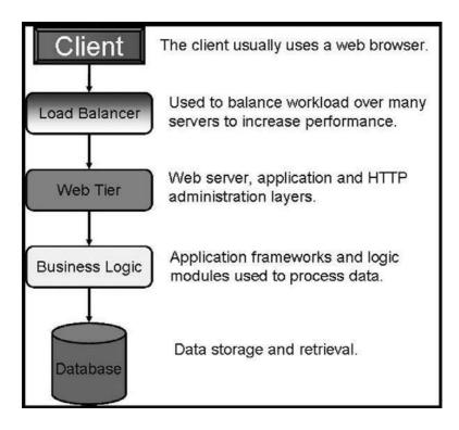
Figure 3.1 The n-tier architecture used in cloud environments.
